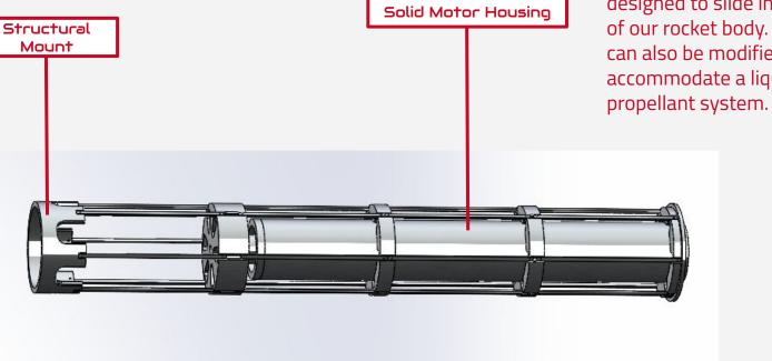
This is our aluminum sled that houses a solid rocket motor. This sled was designed to slide in and out of our rocket body. The sled can also be modified to accommodate a liquid propellant system.
